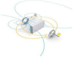
Fig. 2. The power source, left, is connected to AC power. The blue lines represent the magnetic near field induced by the power source. The yellow lines represent the flow of energy from the source to the capture coil, which is shown powering a light bulb. Note that this diagram also shows how the magnetic field (blue lines) can wrap around a conductive obstacle between the power source and the capture device.
