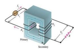
Fig. 3. An electric transformer uses magnetic induction to transfer energy from its primary winding
