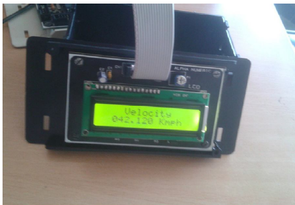
Fig 8 Result display on LCD for an input frequency of 825.88Hz
