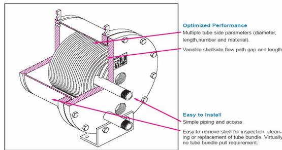
**Fig. 4 Spiral Tube Heat Exchanger**
