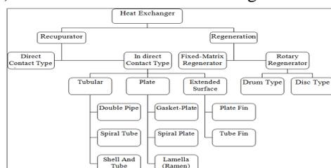
Fig. 1 Classification of Heat Exchangers
