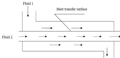
Fig. 2 Double Pipe Heat Exchanger
