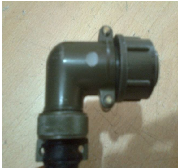
Fig. 1.9 Connector with RTV filled up.
