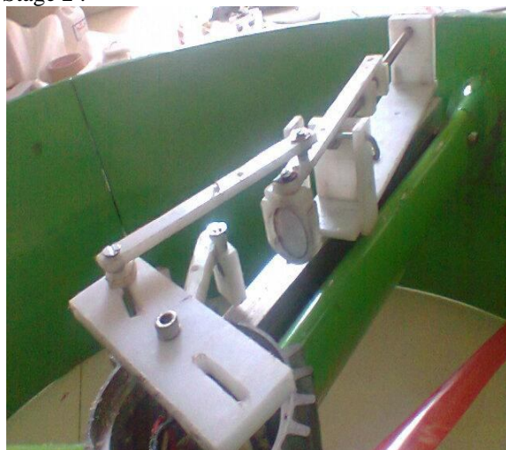
Figure 3 Magnetic acceleration unit at Stage 2 with slot made on the plate
