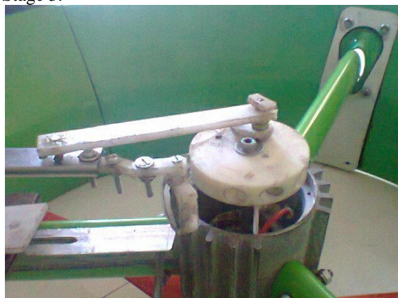
Figure 4 Implementation of the reciprocating motions
