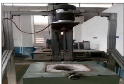
Figure 1: Induction furnace with stirrer arrangement.
