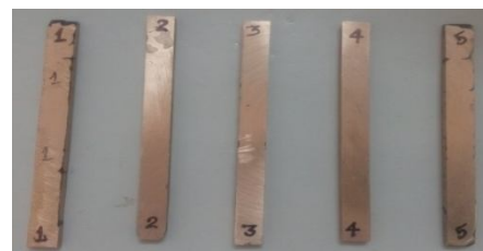
Figure 4 Specimen for 3 point bending test
