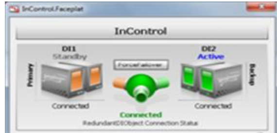
Fig. 11 Connection status of server on failover.
