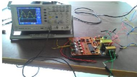
Figure 10: The magnetic inrush current in the hardware on DSO display device
