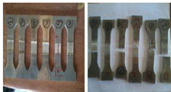
Figure 7: Test specimens before and after tensile test
