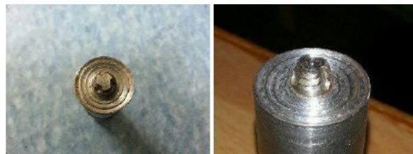
Figure 2: Concave shouldered tool profile design
