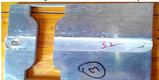
Figure 4 FSW Rotational speed 1400rev/min and transverse speed 100mm/min
