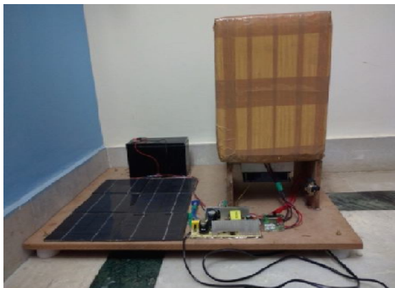
Figure 3: Fabricated Solar Powered Thermoelectric Refrigerator
