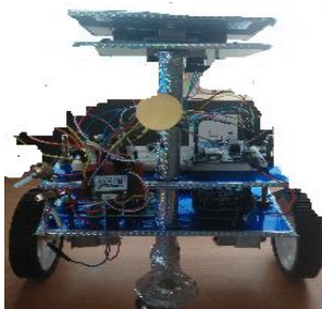
Fig 13. Prototype of smart vehicle using Arduino UNO
