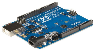
Fig 2. Arduino UNO AT mega328 microcontroller board
